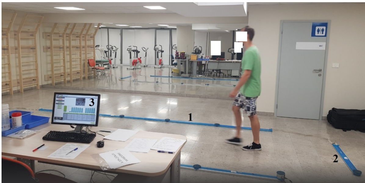
Figure 1: Optogait setup. 1: five 1m transmitting and receiving bars; 2: 2D system for additional gait parameters e.g. gait width; 3: real-time feedback of gait performance representing step lengths.
