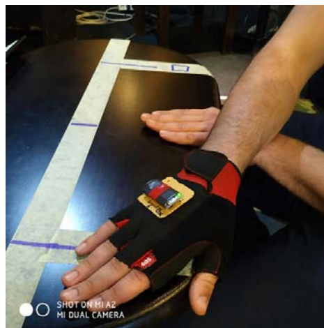
Figure 1. The initial position of the subject's hand with the IMU sensor attached to the glove on Taping test.
